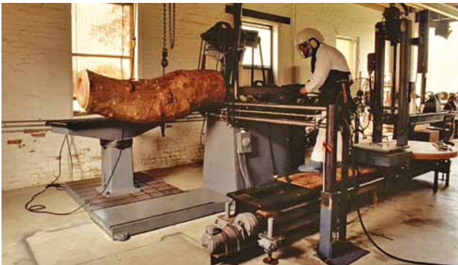
Mark Lindquist with his patternmaker's lathe and his robot ASTRO (assigned specific task robotic operative [extreme right], designed and built by Mark Lindquist).
